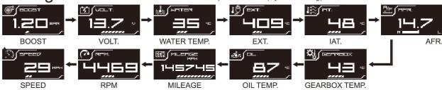
2. Dual mode switching After selecting information 1, you can press the button B to select the required information and then two information can be displayed at the same time.
