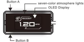
1. Single mode switch Short press button A (Cycle switching)
